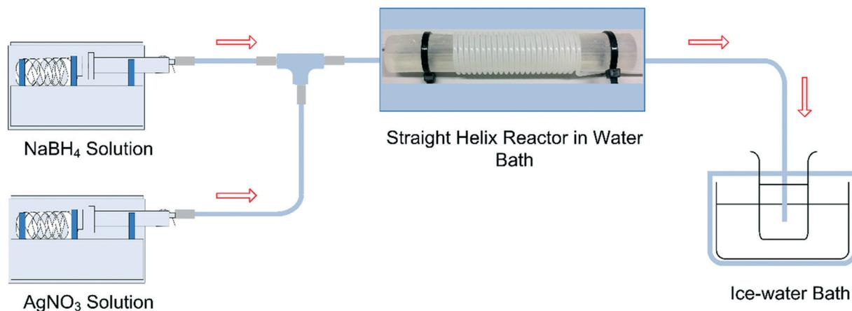
Fig. 1 Schematic diagram of the experimental setup.
