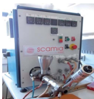
Fig. 7 Representation of a single-screw extruder.
