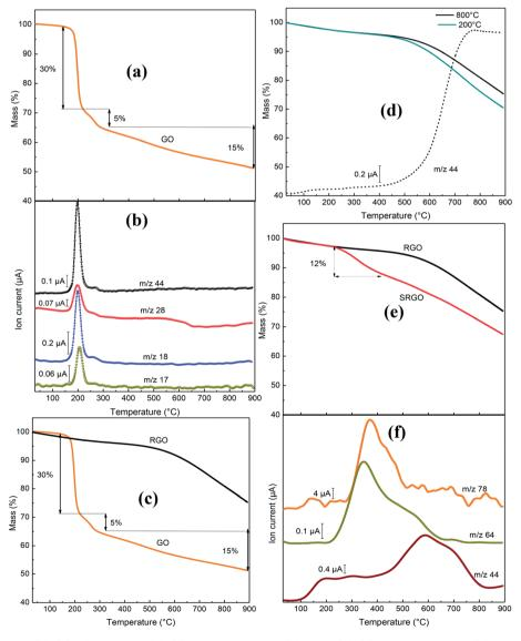
Fig. 8 (a) Mass variation for GO, (b) MS profile for GO, (c) mass variation for GO and RGO, (d) mass variation for GO following heat treatment at 200 and 800  $^{\circ}$ C, MS profile (- - ) for GO following heat treatment at 800  $^{\circ}$ C, (e) mass variation for RGO and SRGO and (f) MS profiles for SRGO.
