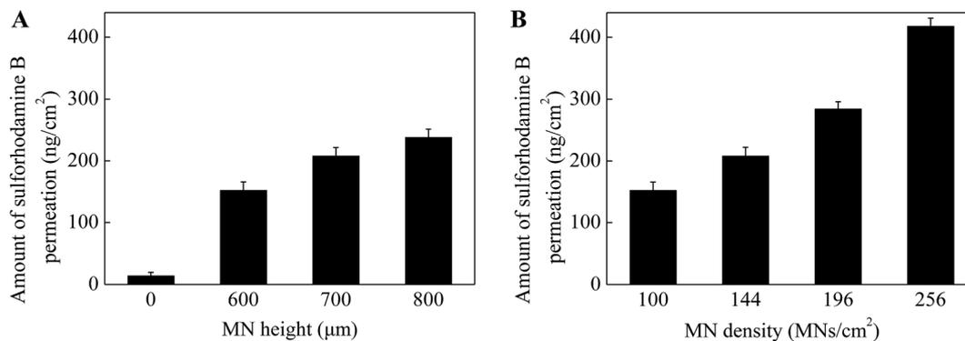
Fig. 3 The amount of sulforhodamine B permeated into the porcine skin treated with MNs with (A) different heights (600, 700 and 800 μm) and (B) densities (100, 144, 196 and 256 MNs per cm<sup>2</sup>) in 5 min from 0.1 mg mL<sup>-1</sup> surforhodamine B solution. Each data point represents the average of 5 experiments. Standard deviation bars are shown.
