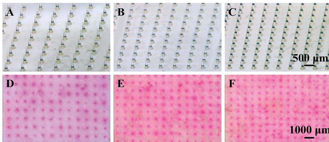
Fig. 4 Microscopic images showing the enlarging structure of the fabricated PLA MNs and the piercing effect of the MNs. (A–C) MN arrays with a height of 600  $\mu\text{m}$  and different densities of (A) 144 MNs per  $\text{cm}^2$ , (B) 196 MNs per  $\text{cm}^2$  and (C) 256 MNs per  $\text{cm}^2$ . (D–F) The porcine skin samples treated with MNs with different densities of (D) 144 MNs per  $\text{cm}^2$ , (E) 196 MNs per  $\text{cm}^2$  and (F) 256 MNs per  $\text{cm}^2$ .
