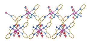
Fig. 4 Crystal structure of  $[PbL(NO_2)]_n$  (hydrogen atoms are omitted for clarity). Tetrel bonds Pb···N and Pb···O are shown as dashed lines. Stronger non-covalent interactions are shown in a darker shade of green than the weaker non-covalent interactions. Color code: C = gold, N = blue, O = red, Pb = magenta.
