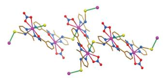
Fig. 6 Crystal structure of  $[Pb_2(HL)_2(NO_3)_2(NCS)_2]$  (CH hydrogen atoms are omitted for clarity). Tetrel bonds Pb···S are shown as dashed lines. Color code: C = gold, H = black, N = blue, O = red, Pb = magenta, S = yellow.
