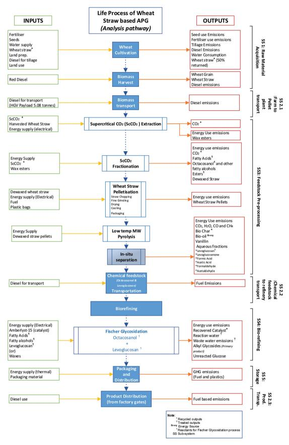
Fig. 1 Cradle-gate life cycle stages for WS-APG production.
