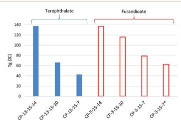
Fig. 5 Effect on the  $T_q$  of co-polymers of isosorbide 15 and co-diols (7, 10 or 14) with 3 (furandioate) and 13 (terephthalate). \*25:75 15:7 molar load ratio.
