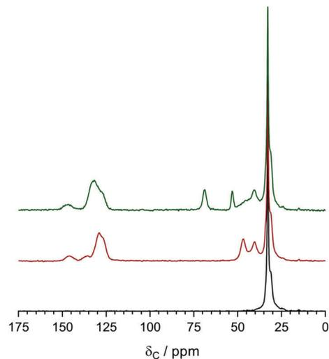
Fig. 6 The <sup>13</sup>C solid-state NMR of the precursor LDPE film (bottom spectrum), the LDPE-*g*-poly(VBC) intermediate film (middle spectrum) and the LDPE-AEM (100 kGy) (top spectrum). Tetramethylsilane was used as the shift reference. Magic angle spinning rotation rate = 10 kHz. All spectra were normalised to the intensity of the  $\delta = 33$  ppm (LDPE-based) peak to aid visual comparison.
