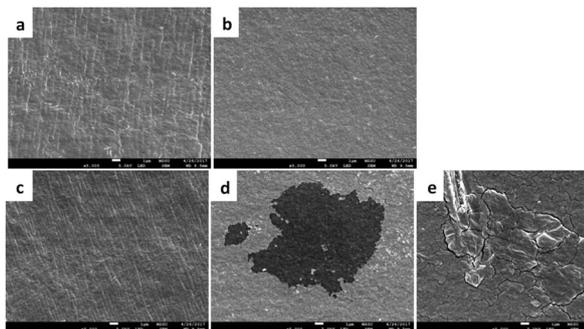
Fig. 11 Scanning Electron Micrographs (SEM) of: (a) pristine LDPE-AEM (100 kGy); (b) pristine ETFE-AEM (30 kGy); (c) LDPE-AEM (100 kGy) degraded in aqueous NaOH (1 mol dm<sup>-3</sup>) for 7 d at 80 °C; (d and e) similarly degraded ETFE-AEM (30 kGy). The white scale bars = 1 μm.
