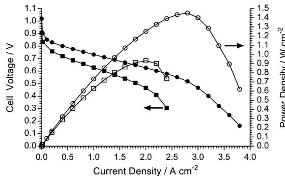
Fig. 14 The H<sub>2</sub>/O<sub>2</sub> AEMFC performances at 80 °C of the LDPE-AEM (100 kGy) with Pt/C (0.4 mg<sub>Pt</sub> cm<sup>-2</sup>) (●,○) and Ag/C (0.8 mg cm<sup>-2</sup>) (■,□) cathodes: PtRu/C (50% wt Pt and 25% wt Ru) anodes (0.4 mg<sub>Pt</sub> cm<sup>-2</sup> loading). The 1.0 SLPM (RH = 100%) gas supplies were not pressurised.
