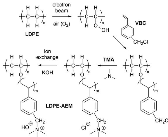
**Scheme 1** An outline of the synthetic process used to synthesise the low-density polyethylene-based anion-exchange membranes (LDPE-AEM). The benchmark ETFE-AEM is synthesised using the same protocol but starting with poly(ethylene-co-tetrafluoroethylene), ETFE, films rather than LDPE.
