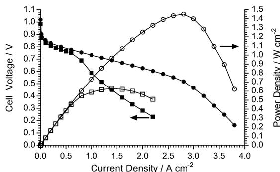
Fig. 13 The AEMFC performances at 80 °C of the LDPE-AEM (100 kGy) with O<sub>2</sub> (●,○) and CO<sub>2</sub>-free air (■,□) supplies as the cathode: PtRu/C (50% wt Pt and 25% wt Ru) anodes and Pt/C (40% wt) cathodes (all 0.4 mg<sub>Pt</sub> cm<sup>-2</sup> loadings). The 1.0 SLPM (RH = 100%) cathode and anode (H<sub>2</sub>) gas supplies were not pressurised.
