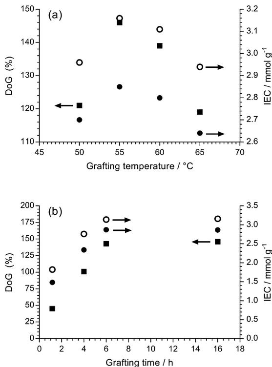
**Fig. 1** (a) The effect of grafting temperature on the degree of grafting (DoG, ■) and the experimental determined ion-exchange capacity (IEC, ●) with a grafting time of 16 h. (b) The effect of grafting time on the DoG and IEC with a grafting temperature of 55 °C. The theoretical ion-exchange capacities (○) are calculated from the experimentally determined DoG values.<sup>24</sup> Grafting mixture: 5% v/v VBC and 1% v/v 1-octyl-2-pyrrolidone dispersed in H<sub>2</sub>O.
