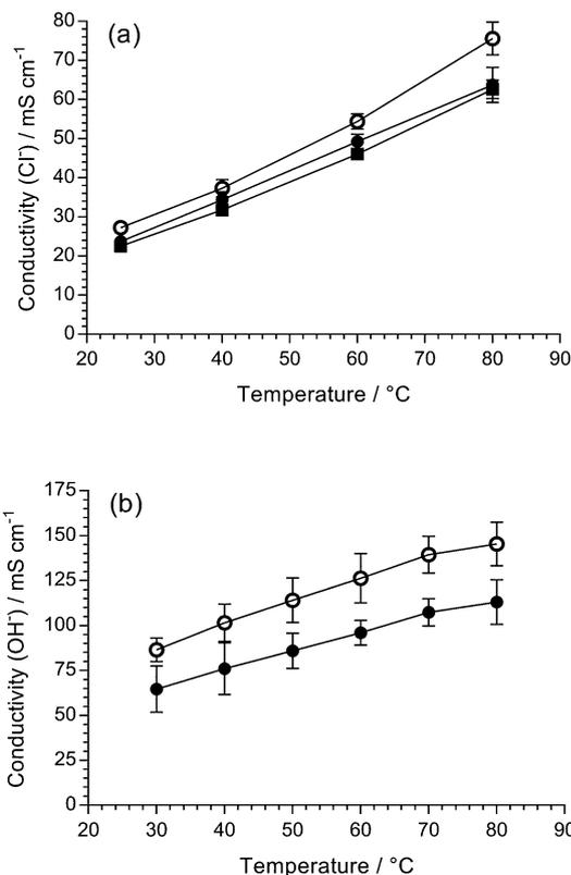
**Fig. 2** (a) The chloride conductivities of fully hydrated ETFE-AEM (30 kGy) (■), LDPE-AEM (50 kGy) (●) and LDPE-AEM (100 kGy) (○) when submerged in UPW. (b) The hydroxide conductivities of LDPE-AEM (50 kGy) (●) and LDPE-AEM (100 kGy) (○) in a RH = 95% CO<sub>2</sub>-free atmosphere. All data from 4-probe (in-plane) measurements. Errors bars = standard deviations from measurements on *n* = 3 samples of each RG-AEM.
