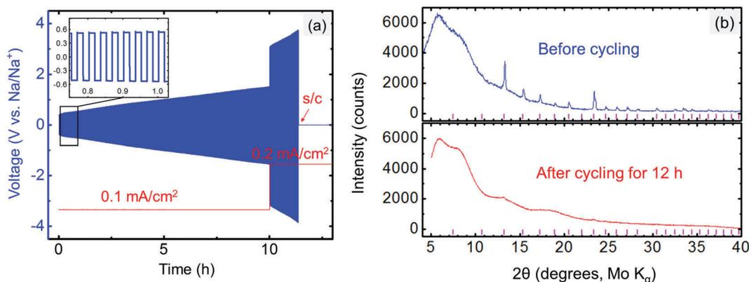
Fig. 8 (a) Electrochemical cycle for Na|Na<sub>3</sub>PSe<sub>4</sub>|Na symmetric cell; a short circuit (s/c) occurred after cycling for 11.4 h. (b) XRD results for Na<sub>3</sub>PSe<sub>4</sub> before and after cycling for 12 h (1 min per cycle); the tick marks indicate Na<sub>3</sub>PSe<sub>4</sub> peaks.
