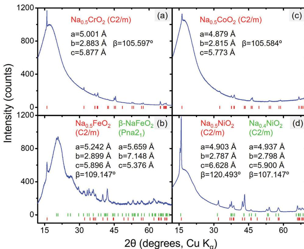
Fig. 5 Diffraction patterns of desodiated compound(s) of (a)  $\text{NaCrO}_2$ , (b)  $\text{NaFeO}_2$ , (c)  $\text{NaCoO}_2$ , and (d)  $\text{NaNiO}_2$ . The peak positions and refined structure data are also displayed; the hump at  $\sim 15^\circ$  in all four figures originates from the Kapton sample holder (the diffraction pattern of the empty sample holder is presented in Fig. S3, ESI†).
