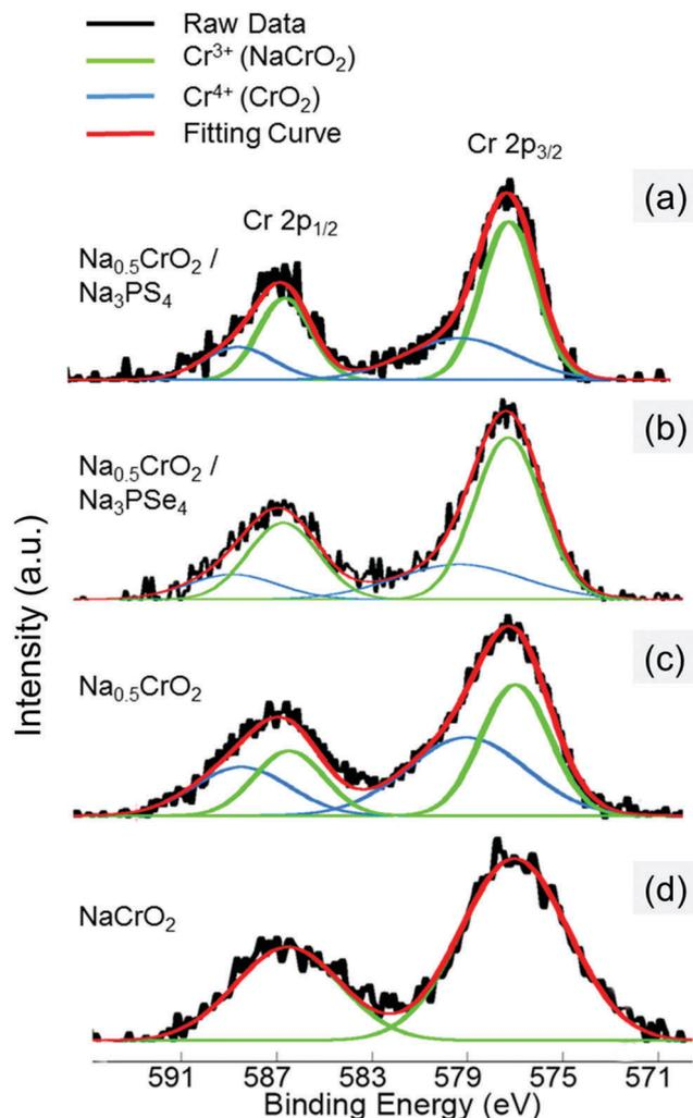
Fig. 7 XPS spectra of Cr 2p from the surfaces of (a) mixture of  $\text{Na}_{0.5}\text{CrO}_2$  and  $\text{Na}_3\text{PS}_4$  at RT ( $25^\circ\text{C}$ ), (b) mixture of  $\text{Na}_{0.5}\text{CrO}_2$  and  $\text{Na}_3\text{PSe}_4$  at RT ( $25^\circ\text{C}$ ), (c)  $\text{Na}_{0.5}\text{CrO}_2$ , and (d)  $\text{NaCrO}_2$ .
