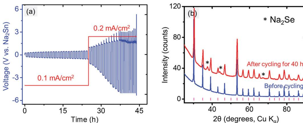
Fig. 9 (a) Electrochemical cycling of Na<sub>2</sub>Sn|Na<sub>3</sub>PSe<sub>4</sub>|Na<sub>2</sub>Sn symmetric cell. (b) XRD patterns of Na<sub>3</sub>PSe<sub>4</sub> before and after cycling for 40 h (60 min per cycle); the tick marks indicate Na<sub>3</sub>PSe<sub>4</sub> peaks.
