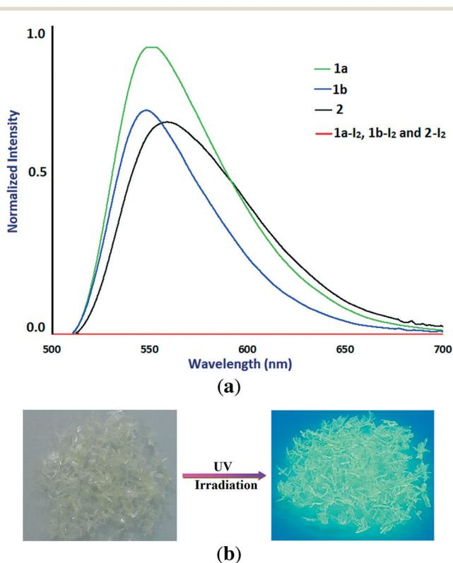
**Fig. 8** (a) Solid-state luminescence spectra of **1a** (green), **1b** (blue) and **2** (black) at room temperature ( $\lambda_{\text{ex}} = 300$  nm) before and after iodine sorption (red). (b) Crystals of **1a** under UV irradiation at 254 nm at room temperature.
