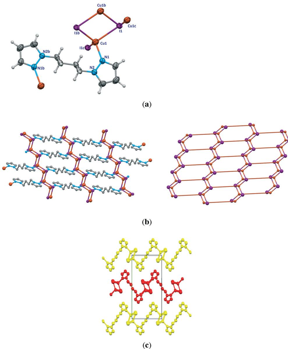
**Fig. 1** The structure of  $[\text{Cu}_2(\mu_3\text{-I})_2(\mu\text{-bpb})]_n$  (**1a**). (a) Asymmetric unit of **1a** with additional atoms to complete the bpb ligand and the coordination of Cu and I. (b) 2D polymeric structure with parallel staircase  $[\text{Cu}_2\text{I}_2]_n$  units and the underlying net **bey**. (c) View of the ABAB packing modes of three parallel undulating sheets along the  $[1\ 0\ 0]$  direction.
