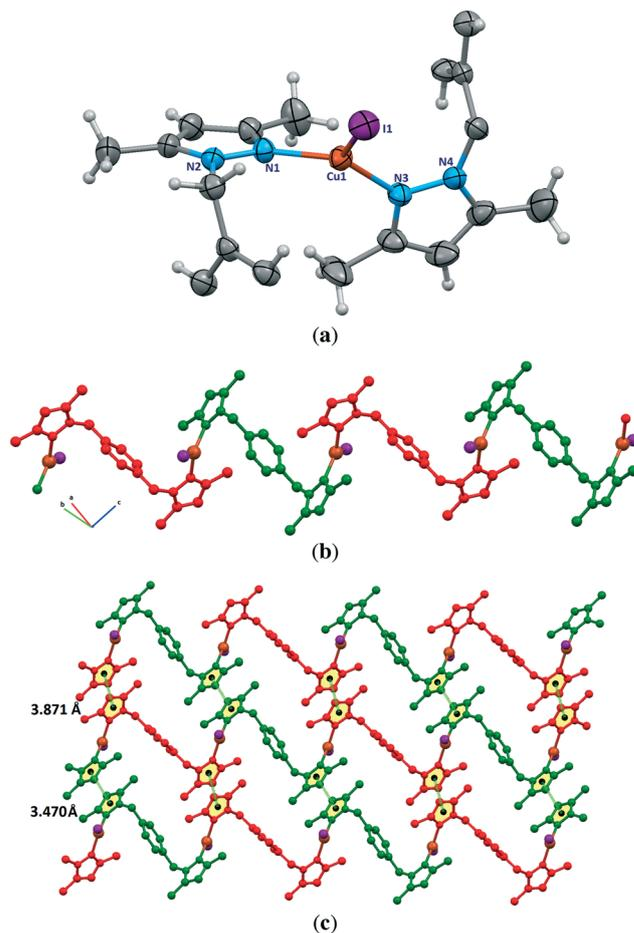
Fig. 5 The structure of  $[\text{CuI}(\mu\text{-bdb})]_n$  (**3**). (a) Asymmetric unit of **3** with labeling scheme for non-H and C atoms. (b) 1D zigzag structure of **3** containing a sequence of  $\mu\text{-bdb}$  ligands with two different conformations. (c)  $\pi\cdots\pi$  stacking interactions between the chains giving 2D supramolecular layers.
