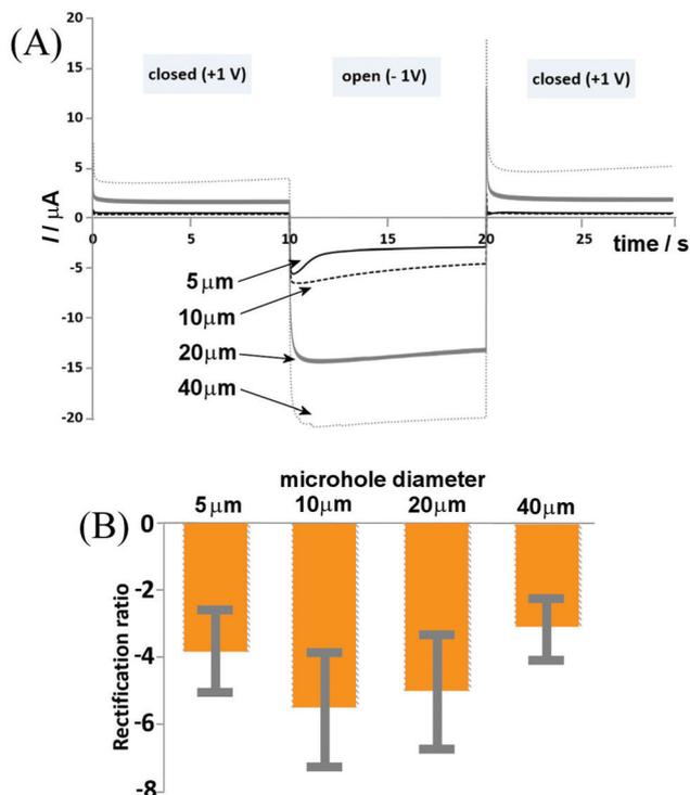
**Fig. 7** (A) Chronoamperometry transient data for chitosan-doped cellulose film diodes switching between +1 V (closed state) and -1 V (open state) for PET microholes of 5, 10, 20, and 40  $\mu\text{m}$  diameter immersed in 50 mM NaCl. (B) Bar plot of rectification ratios as a function of microhole diameter. Errors are estimated as  $\pm 30\%$  to account for some variations in the film formation.
