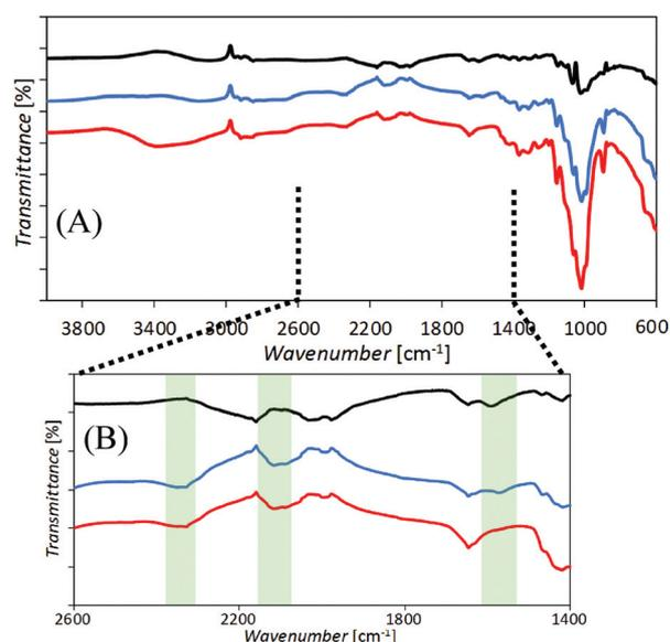
**Fig. 3** (A, B) FTIR spectra of chitosan (black line); cellulose (red line); and cellulose–chitosan blend (blue line) bulk films cast for analysis. Signals unique to both cellulose (2400–2300  $\text{cm}^{-1}$  and 2160–2040  $\text{cm}^{-1}$ ) and chitosan (1600–1550  $\text{cm}^{-1}$ , attributable to N–H bonds) are present in the co-deposited films, confirming the presence of both polymers.
