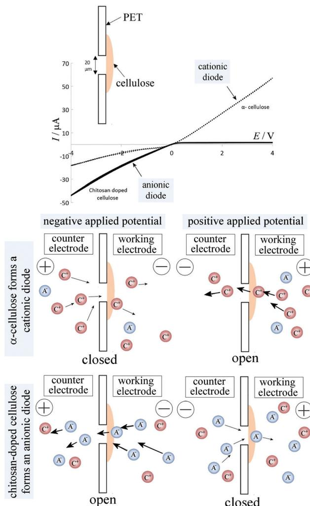
**Fig. 5** Cyclic voltammetry (scan rate: 20  $\text{mV s}^{-1}$ ) of  $\alpha$ -cellulose only films (dotted line) and chitosan-doped PET cellulose films (black solid line) on a 20  $\mu\text{m}$  diameter microhole in a PET sheet in 50 mM NaCl on both sides of the membrane. The schematic drawing shows the four mechanistic cases of a cationic diode and an anionic diode under positive potential and negative potential polarisation, respectively.
