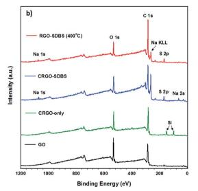
Fig. 2 (a) ATR-FTIR and (b) XPS survey spectra of GO, CRGO-only, with SDBS and thermally reduced CRGO-SDBS (RGO-SDBS).
