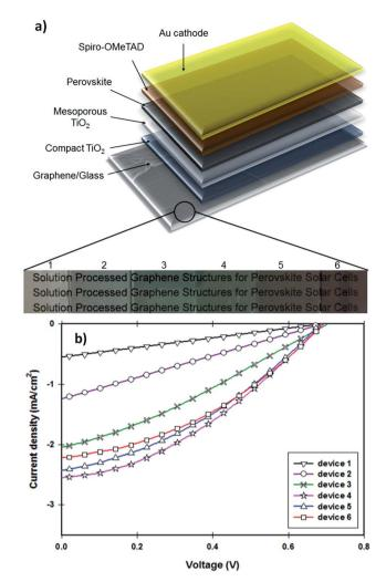
Fig. 5 (a) Device structure, (b) photocurrent density–voltage (J-V) curve of the fabricated solar cells with transparent graphene electrodes. PSC devices with 0.075 cm<sup>2</sup> active area were illuminated under AM 1.5G simulated sunlight (100 mW cm<sup>-2</sup>).
