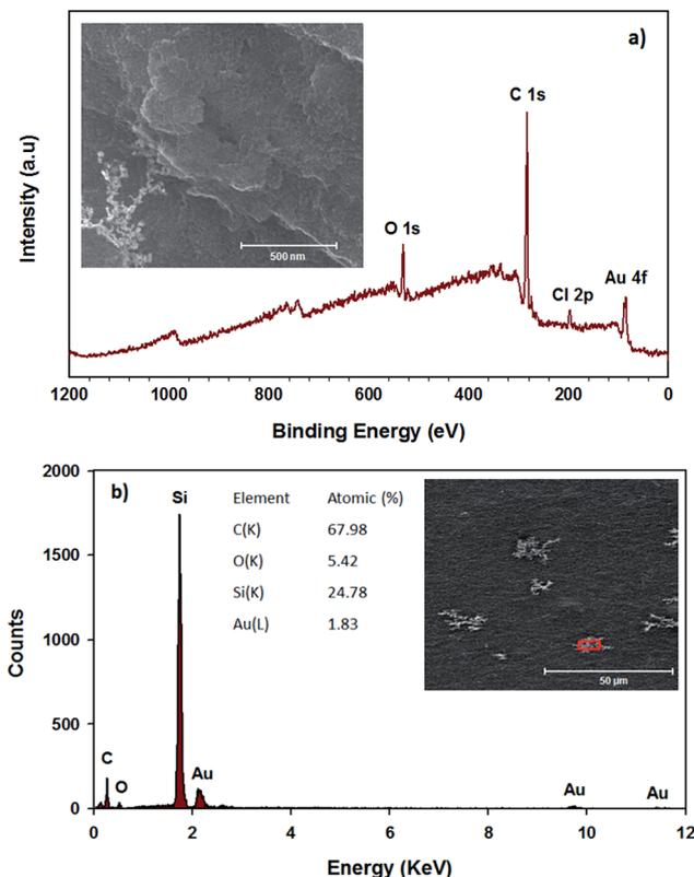
Fig. 3 (a) XPS survey spectra (inset: SEM image of AuNPs–RGO) and (b) EDX analysis (red box in the inset is the selected area for analysis) of RGO–SDBS film after HNO<sub>3</sub> and HAuCl<sub>4</sub> treatments.
