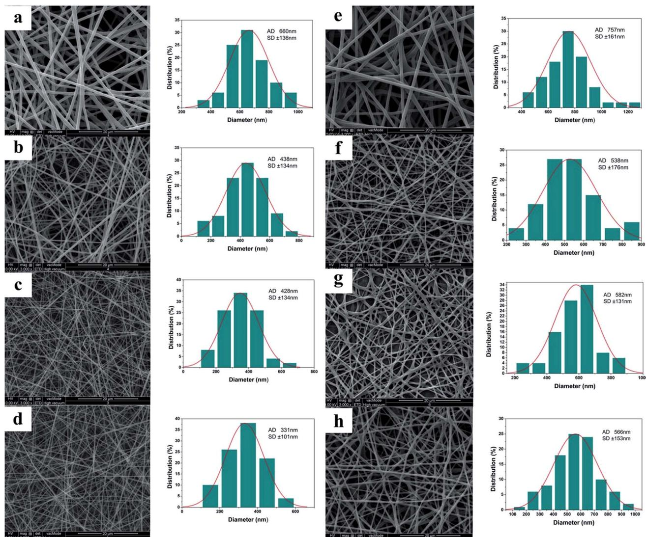
Fig. 1 SEM images and diameter distributions of electrospun nanofibers prepared with (a) pure gelatin (G); (b) gelatin and VA (G/A); (c) gelatin and VE (G/E); (d) gelatin, VA and VE (G/A + E); and the same fibers after cross-linking: (e) G; (f) G/A; (g) G/E; (h) post-crosslinking G/A + E.
