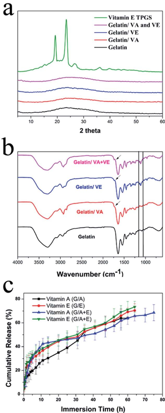
Fig. 3 (a) XRD patterns of vitamin E TPGS and the cross-linked nanofibers prepared in this work; (b) FTIR spectra of the cross-linked fibers; (c) the *in vitro* vitamin release profiles from the G/A, G/E and G/A + E fibers.
