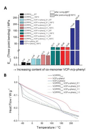
Fig. 4 (A) Determined E-moduli of cured VCPPPG $_{2000}$  and VCPP-m-phenyl specimens, as well as by co-networks in ratios of 6:1 and 1:1 of VCPPPG $_{2000}$ , VCPP-m-phenyl and VCPP-p-phenyl. With increasing content of the co-monomer VCP-m/p-phenyl, the moduli could be raised up to 1200 times to higher values. (B) Second DSC heating trace of cured VCP specimens, illustrating the glass transition  $T_g$  of the cured samples.
