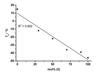
Fig. 3 Linear correlation between the measured  $T_gs$  (from DSC) and the mol fraction of (2) in the copolymers  $P(1_x-co-2_y)_n$ .
