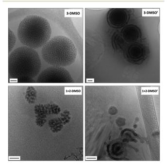
Fig. 2 Representative cryo-TEM images of self-assemblies 3-DMSO with a concentration of 1 mg mL $^{-1}$  and its annealed sample 3-DMSO' at 0.2 mg mL $^{-1}$ ; 1 + 2-DMSO at a concentration of 1 mg mL $^{-1}$  and its annealed sample 1 + 2-DMSO' at 0.2 mg mL $^{-1}$ . Scale bar: 100 nm.
