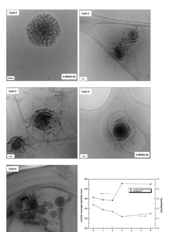
Fig. 5 Evolution of self-assembly from 3-DMSO to 3-DMSO' with 6 annealing cycles characterized by cryo-TEM analysis (scale bar = 50 nm) and the number-average diameter and size distributions determined by DLS analysis.
