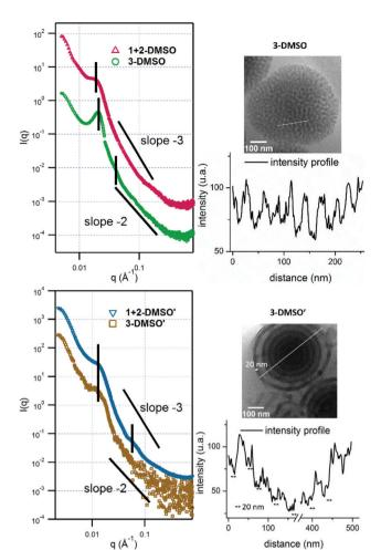
Fig. 3 SAXS profiles of self-assemblies 3-DMSO, 1 + 2-DMSO, 3-DMSO', and 1 + 2-DMSO'. The vertical black lines indicate the major peaks, indicative of the internal structure of the assemblies. The 1 + 2-DMSO and 1 + 2-DMSO' curves have been shifted by a factor 10 to improve clarity. Cryo-TEM images of 3-DMSO and 3-DMSO' and the corresponding intensity profile along the white line on the TEM images.
