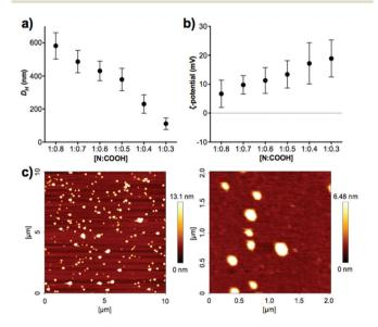
Fig. 2 (a) Hydrodynamic diameter ( $D_{\rm H}$ ) and (b) ζ-potential of P1<sub>SH</sub> PIC nanoparticles prepared at different N:COOH ratios. (c) AFM characterisation of PIC nanoparticles prepared at a 1:0.3 N:COOH ratio.  $D=127\pm42$  nm, n=48.
