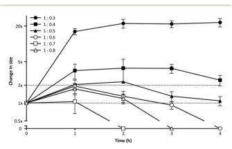
Fig. 3 Relative change in size for  $P1_{SH}$  PIC nanoparticles prepared at different N:COOH ratios and incubated under simulated physiological conditions (154 mM NaCl, pH 7.4, 37 °C). Particle size was normalised to that of a control in the absence of NaCl (1x). n=3.
