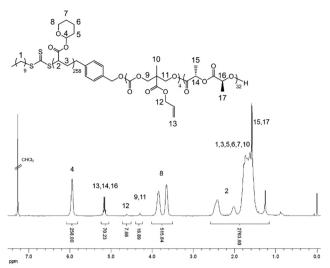
Fig. 1  $\,^{1}$ H NMR spectrum (400 MHz, CDCl $_{3}$ ) of PLLA-b-PMAC-b-PTHPA triblock copolymer, 4.
