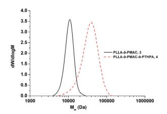
Fig. 2 SEC chromatograms (CHCl $_3$  with 0.5% TEA as eluent, RI detection) of PLLA-b-PMAC diblock copolymer, 3 and PLLA-b-PMAC-b-PTHPA triblock copolymer, 4.
