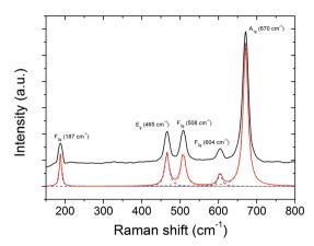
Fig. 8 Raman spectrum of the sample prepared upon pyrolysis of poly(CpCoCbMA) at 800 °C under a nitrogen atmosphere showing the five Raman-active optical-phonon modes of spinel-type Co<sub>3</sub>O<sub>4</sub>.
