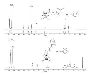
Fig. 3 <sup>1</sup>H NMR spectra and signal assignment of the cobalt-methacrylate monomer 5 (CpCoCbMA) (top) and of a corresponding poly (CpCoCbMA) obtained upon thermal polymerization of 5 (bottom).
