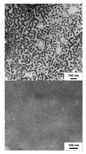
Fig. 10 TEM images of PMMA-block-PCpCoCbMA micelles formed in chloroform after treatment with decamethylcobaltocene ( $Cp_2*Co$ ) (top) or treatment with NOBF<sub>4</sub> (bottom). The micelles were deposited on a carbon-coated copper grid followed by drying at ambient temperature. Scale bars correspond to 100 nm.
