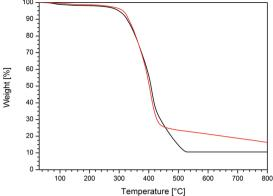
Fig. 6 TGA curves of poly(CpCoCbMA) performed with a heating rate of 10 K min<sup>-1</sup> starting from room temperature to 800 °C under oxygen (black curve) and nitrogen (red curve) atmospheres
