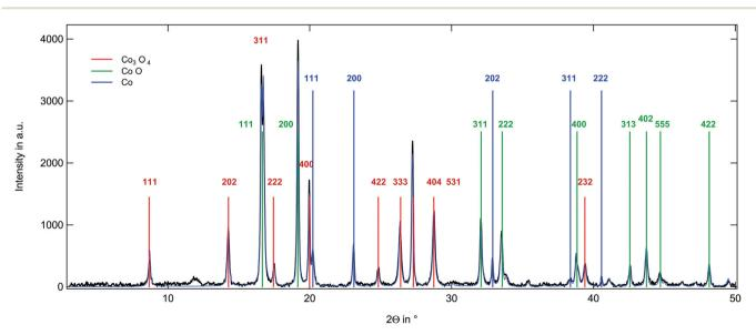
Fig. 7 XRD pattern on the magnetic material obtained by thermal treatment of poly(CpCoCbMA) samples under a nitrogen atmosphere at 800 °C (see the text).
