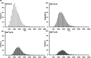
Fig. 4 ESI-TOF mass spectrum of PBC 7 (Table 2, entry 7) terminated with the hydroxyl group, (a) complete spectrum and a part of the spectrum distinguished by carrying charges a = 1, 2, 3 and 4 in the region m/z 400 to 2500, and (b) separated spectra with a = 1, 2, 3 and 4.
