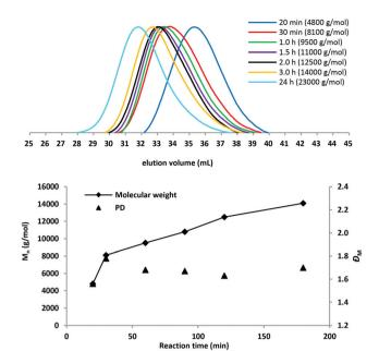
Fig. 3 SEC traces and plot  $M_n$  (determined by SEC) and the dispersity values of PBC 9 versus the polymerization time in the 2nd step.
