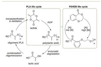
Scheme 2 Idealized life cycles of poly(lactic acid) and poly(2-(2-hydro-xyethoxy)benzoate) moving from four energy intensive steps in PLA recycling to simple ring-opening polymerization and ring closing depolymerization steps for P2HEB.
