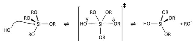
Scheme 2 Base catalysed hydrolysis of silicon alkoxides.
