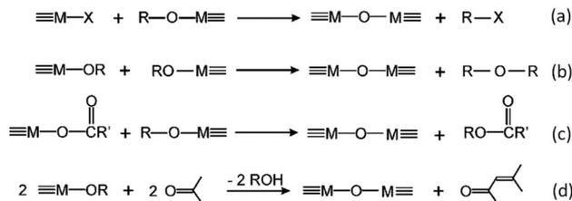
**Scheme 6** Condensation steps in non-hydrolytic sol-gel chemistry including (a) alkyl halide elimination, (b) ether elimination, (c) ester elimination and (d) aldol-like condensation. Modified with permission from ref. 133.
