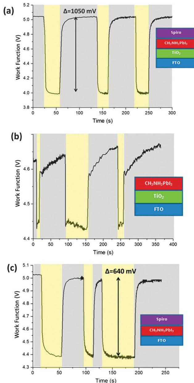
**Fig. 3** Light response of different stacks. In the yellow regions the light is on, while in the grey regions the light is off. (a) Shows the light response of a completed solar cell stack, (b) shows a stack with the spiro-OMeTAD layer omitted, and (c) shows a stack with the TiO<sub>2</sub> omitted. The data is corrected from raw data to give absolute work function.
