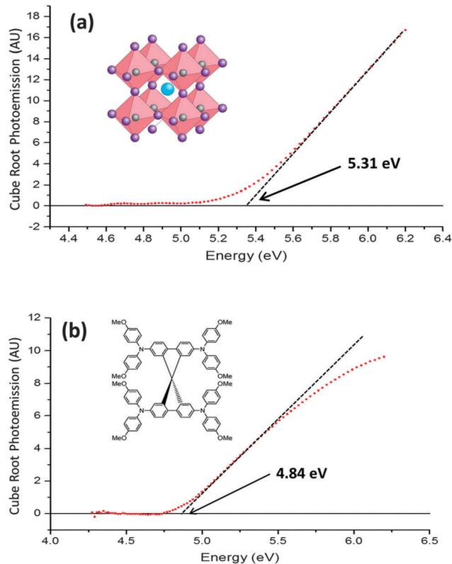
Fig. 2 (a) Ambient pressure photoemission spectroscopy data for  $\text{CH}_3\text{NH}_3\text{PbI}_3$  on an FTO substrate. (b) Ambient pressure photoemission spectroscopy data for spiro-OMeTAD on an FTO substrate. The HOMO levels are determined by extrapolating the linear part of the curve down to the baseline signal level. The structures of the materials are shown in the inset of their respective graphs.
