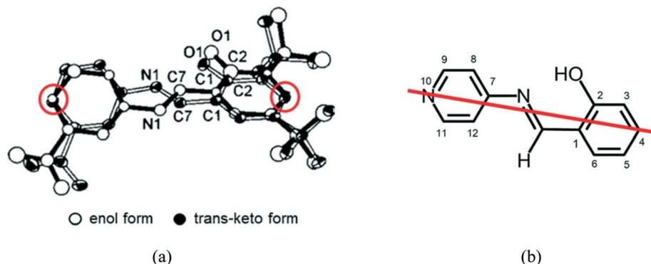
Fig. 12 (a) Observed structure of the *trans*-keto form of SA,<sup>6</sup> and (b) the model structure of the *trans*-keto form of SAP, assuming that the pedal motion occurs keeping the carbon atom 4 and the nitrogen atom 10 in the same positions.
