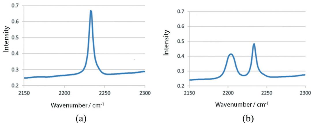
Fig. 4 Change in IR spectra of I (a) before and (b) after 120 min visible-light irradiation. The stretching vibration modes of the 2-ce and 1-ce groups appear at 2240 and 2200  $\text{cm}^{-1}$ , respectively.
