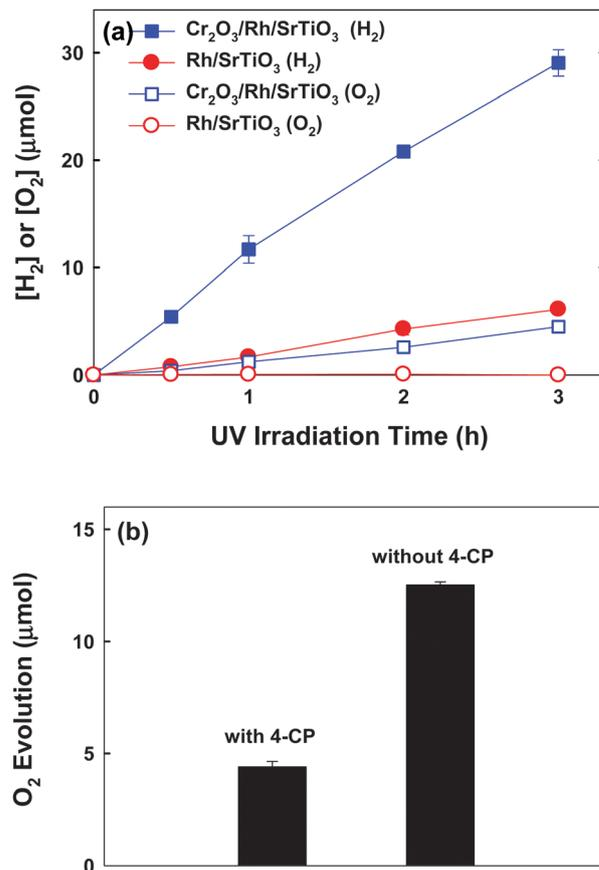
Fig. 2 (a) Time-profiled production of H<sub>2</sub> and O<sub>2</sub> in the suspension of Cr<sub>2</sub>O<sub>3</sub>/Rh/SrTiO<sub>3</sub> and Rh/SrTiO<sub>3</sub> with 4-CP (300 μM) in the initially de-aerated suspension. (b) Comparison of photocatalytic O<sub>2</sub> evolution in the suspension of Cr<sub>2</sub>O<sub>3</sub>/Rh/SrTiO<sub>3</sub> (after 3 h reaction) in the presence and absence of 4-CP.
