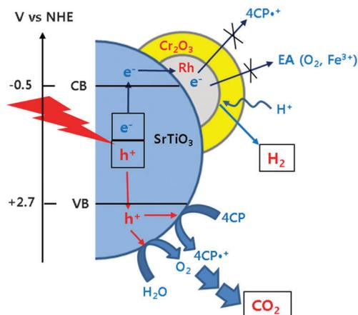
**Scheme 1** Schematic illustrations of photocatalytic reaction mechanisms occurring on the surface of  $\text{Cr}_2\text{O}_3/\text{Rh}/\text{SrTiO}_3$ .
