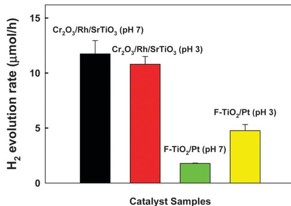
Fig. 3 Comparison of the initial photocatalytic H<sub>2</sub> production rate between Cr<sub>2</sub>O<sub>3</sub>/Rh/SrTiO<sub>3</sub> and F-TiO<sub>2</sub>/Pt photocatalytic systems in the presence of 4-CP (300 μM). Experimental conditions: [catalyst] = 0.5 g L<sup>-1</sup>, λ > 320 nm, air-tight and initially Ar-purged for 1 h before UV irradiation.
