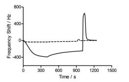
Fig. 4 Frequency responses of protein binding and sensor surface regeneration. Anti-biotin  $F_{ab}$  binding to biotin-derivatized pAAc surface (—); anti-biotin  $F_{ab}$  binding to biotin-derivatized carboxyl-terminated SAM surface (---). Sample concentrations: 25  $\mu$ g mL<sup>-1</sup>; flow rate: 25  $\mu$ L min<sup>-1</sup>. Surfaces were regenerated with glycine (10 mM, pH 1.5).
