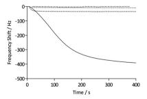
Fig. 3 Frequency responses of protein binding to QCM sensors. Antibiotin F<sub>ab</sub> binding to biotin-derivatized pAAc surface (-); anti-biotin F<sub>ab</sub> binding to biotin-derivatized carboxyl-terminated SAM surface (---); anti-biotin Fab binding to deactivated pAAc surface (---); lysozyme binding to biotin-derivatized pAAc surface (\*\*\*). Sample concentrations: 25  $\mu$ g mL<sup>-1</sup>; flow rate: 25  $\mu$ L min<sup>-1</sup>.
