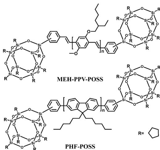
Fig. 14 Chemical structures of MEH-PPV-POSS and PHF-POSS.
