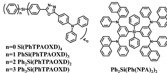
Fig. 1 Chemical structures of tetraphenylsilane derivatives functionalized with triphenylaminooxadiazole and diarylamine.
