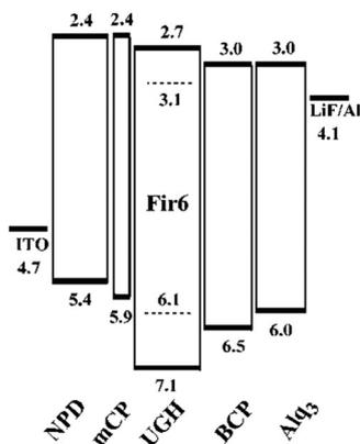
Fig. 3 The energy level diagram (units: eV) for the device: ITO/NPD (400 Å)/mCP (100 Å)/Fir6:UGH (10%, 250 Å)/BCP (150 Å)/Alq<sub>3</sub> (250 Å)/LiF/Al. Reproduced with permission from ref. 47. Copyright 2004 American Chemical Society.
