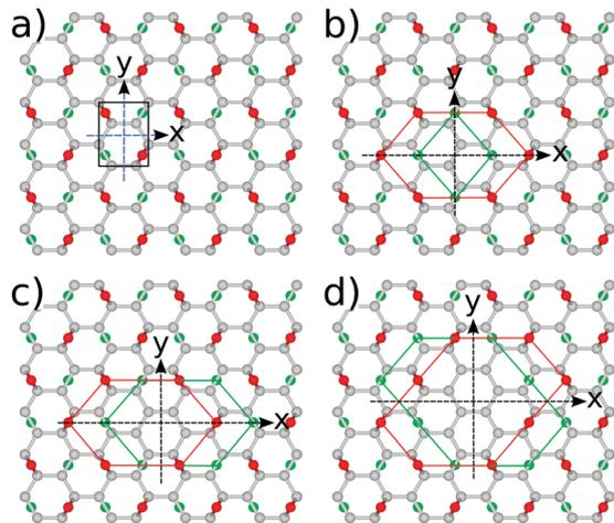
Fig. 9 Symmetries of several representative unit cell structures: (a) fully oxidized graphene surface,  $C_{2v}$ , (b) single O vacancy,  $C_{2v}$ , (c) two vacancies,  $C_{2v}$ , and (d) four O vacancies,  $C_{2v}$ . All arrangements in unit cells with  $n_v \neq 0$  corresponding to those with minimal energy.
