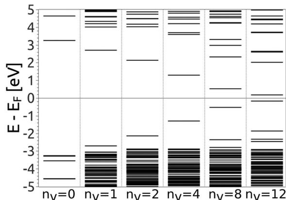
Fig. 5 Evolution of the electronic structure change and the energy gap with the increase of the number of O vacancies,  $n_v$ . On the left side the electronic states at the  $\Gamma$  point of the fully oxidized graphene are also presented. All results are obtained by the PBE0 exchange correlation functional.
