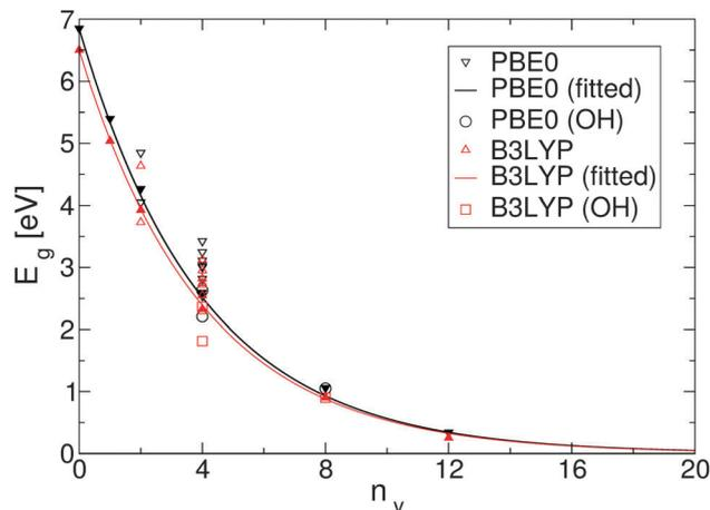
Fig. 4 Dependence of the fundamental energy gap as a function of the number of O vacancies,  $n_v$ . For  $n_v = 2$  and  $n_v = 4$  energy gaps for all possible configurations are depicted. Solid lines are fits through the calculated values for most stable structures. Circles and squares represent structures with added hydroxyl groups.
