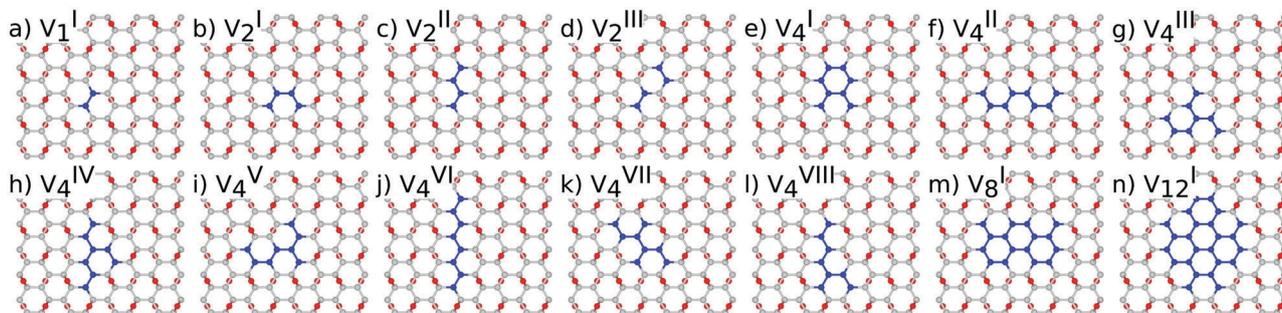
**Fig. 3** Atomic structure of the 96 carbon atom sub-lattice and  $n_v$  oxygen vacancies of the unit cell: (a)  $n_v = 1$ , (b–d)  $n_v = 2$ , (e–l)  $n_v = 4$ , (m)  $n_v = 8$ , and (n)  $n_v = 12$ . For  $n_v = 8$  and  $n_v = 12$  only the most stable structure is presented. The superscript in  $V_{n_v}^I$  represents different topologies with the same  $n_v$ . Carbon atoms that do not form part of functional groups coloured green for clarity.
