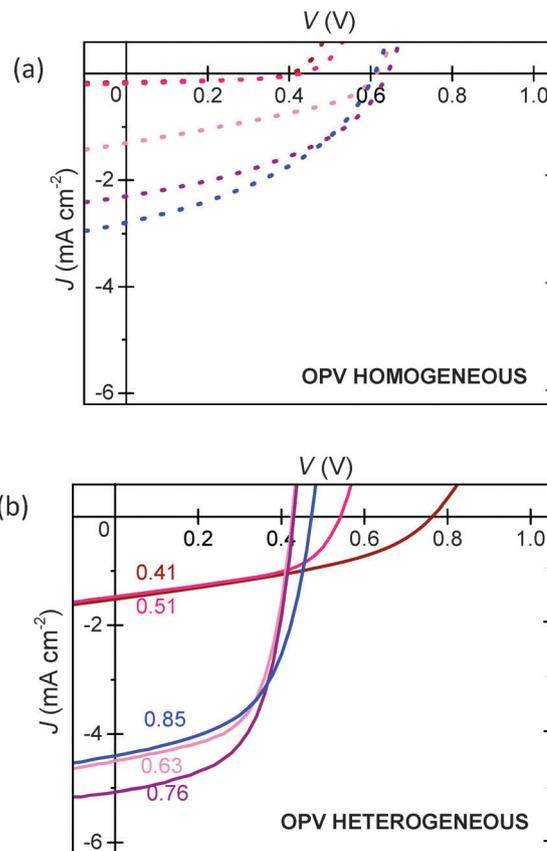
Fig. 6  $J$ - $V$  characteristics of (a) homogeneous and (b) heterogeneous P3HT:PCBM OPVs under AM1.5 illumination with various blend ratios:  $p_{P3HT} = 0.41$  (brown), 0.51 (red), 0.63 (pink), 0.76 (purple) and 0.85 (blue).
