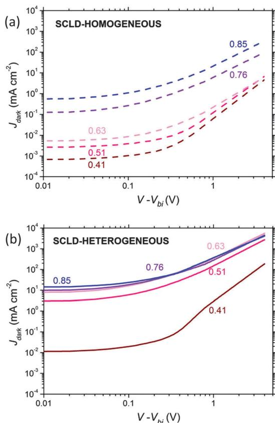
Fig. 2  $J$ - $V$  characteristics under dark conditions for hole-only SCLD P3HT:PCBM diodes for (a) homogeneous and (b) heterogeneous active layers, and blend ratios:  $p_{\text{P3HT}} = 0.41$  (brown), 0.51 (red), 0.63 (pink), 0.76 (purple) and 0.85 (blue).
