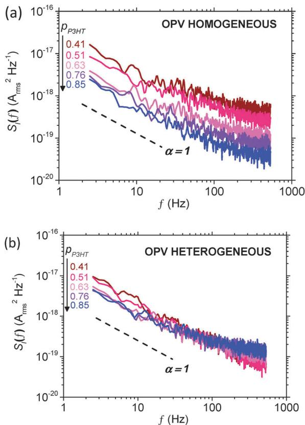
Fig. 7  $1/f$  noise spectra for (a) homogeneous and (b) heterogeneous P3HT:PCBM OPVs with various blend ratios:  $p_{\text{P3HT}} = 0.41$  (brown),  $0.51$  (red),  $0.63$  (pink),  $0.76$  (purple) and  $0.85$  (blue).
