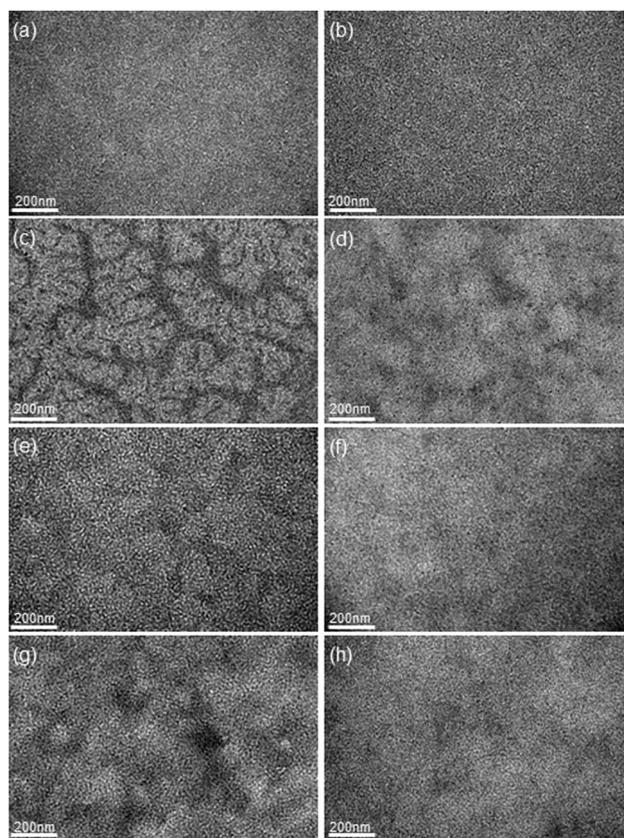
Fig. 1 TEM images of the P3HT:PCBM blends: (a) and (b)  $p_{P3HT} = 0.41$ , (c) and (d)  $p_{P3HT} = 0.51$ , (e) and (f)  $p_{P3HT} = 0.63$ , (g) and (h)  $p_{P3HT} = 0.85$ ; with thermal treatments: left column (a)–(g) corresponds to heterogeneous active layers, while right column (b)–(h) corresponds to homogeneous active layers.
