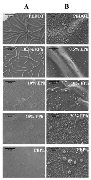
Fig. 6 SEM images of P(EDOT-co-EPh) films as a function of EPh feed ratio; (A) column: lower magnification (scale bar represents 50 μm); (B) column: higher magnification (scale bar represents 5  $\mu$ m).
