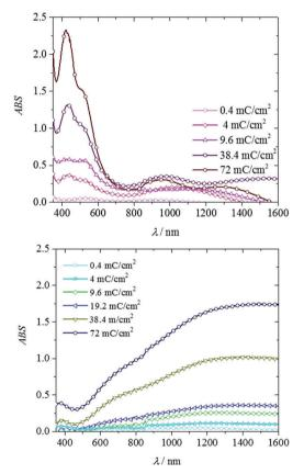
Fig. 5 UV-vis-NIR spectra of polymers at different deposition charges. Top: PEPh; bottom: PEDOT
