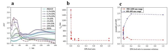
Fig. 4 (a) UV-vis-NIR absorption of the PEDOT-co-EPh copolymers; (b)  $\lambda_{max}$  versus composition; (c) normalized absorption in near-infrared (900-1600 nm) and visible (400-600 nm) wavelength range versus composition.
