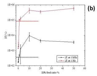
Fig. 7 (a) Impedance amplitude of PEDOT and PEDOT-co-EPh copolymers as a function of frequency; (b) impedance amplitude at 1 Hz and 1 kHz for the PEDOT-co-EPh copolymers as a function of EPh content; dashed lines indicate the impedance amplitude of bare Pt electrode at 1 Hz (red) and 1 kHz (black), respectively (deposition charge: 288 mC cm<sup>-2</sup>).
