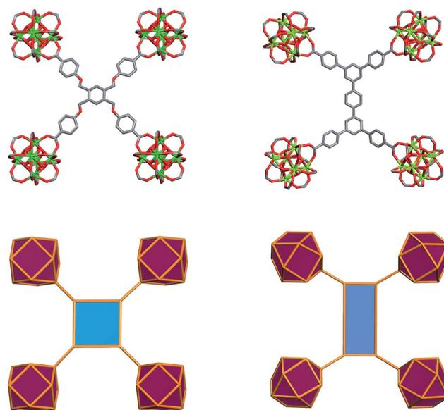
Fig. 5 Illustration of the ligand geometry effect on the orientation of the 12-c cluster in **ftw**-fragment of **ftw**-MOF-1 (left) and **ftw**-MOF-2 (right).<sup>11</sup>
