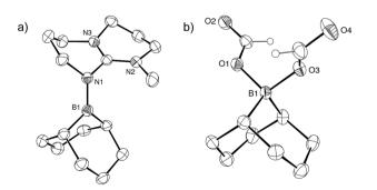
Fig. 1 (a) ORTEP view of 2<sup>+</sup> in [2<sup>+</sup>, I<sup>-</sup>]. Displacement ellipsoids are drawn at the 50% probability level. Counterion and hydrogen atoms are omitted. (b) ORTEP view of compound 5<sup>-</sup> in [TBDH<sup>+</sup>, 5<sup>-</sup>]. Displacement ellipsoids are drawn at the 30% probability level. TBDH<sup>+</sup> and hydrogen atoms on the BBN bicycle have been removed for clarity.
