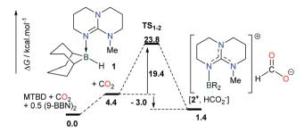
Scheme 1 Computed pathway (M05-2X/6-31+G\*) in THF for the rate-determining step in the MTBD-catalyzed hydroboration of CO<sub>2</sub> to formate.
