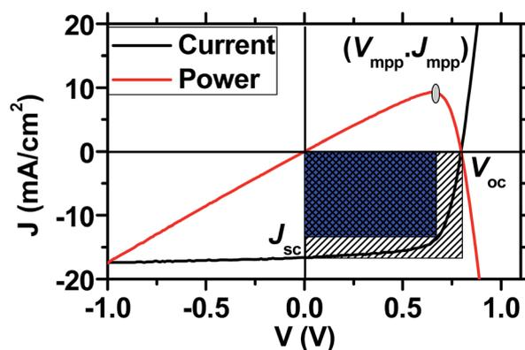
Fig. 6 Typical current-density–voltage ( $J$ - $V$ ) characteristics (black) and the relative output electric power–voltage curve (red) from a BHJ solar cell under illumination by an AAA-grade AM1.5G simulator.
