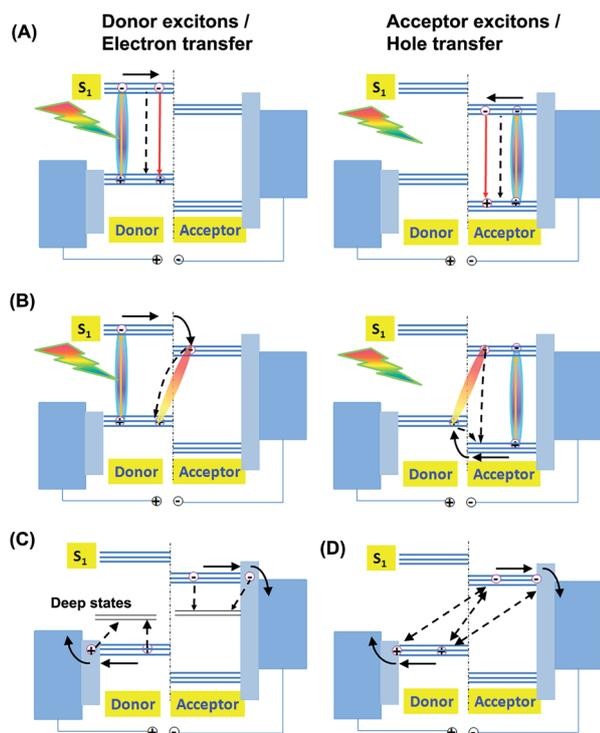
Fig. 7 Schematic depictions of the generation of donor excitons and acceptor excitons, electron and hole transfer, and loss mechanisms *via* exciton decay (A), recombination of bound electron-hole pairs (B), and recombination of mobile electrons and holes as trapped by deep states (C) or in a bimolecular mechanism (D).
