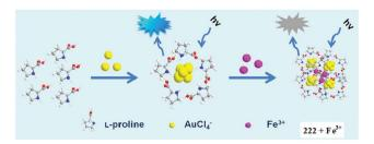
Fig. 186 Schematic of the formation and  ${\rm Fe}^{3+}$ -mediated fluorescence quenching of AuNCs 222.
