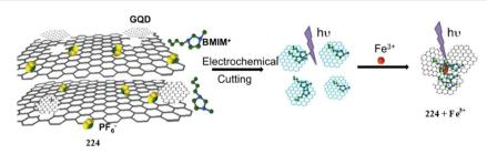
Fig. 188 Schematic of graphene quantum dots (GQD) synthesis from 3D graphene and the mechanism of Fe<sup>3+</sup> detection.
