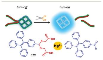
Fig. 289 Schematic of the polarity dependent chemosensor 329 for  $Hq^{2+}$ .
