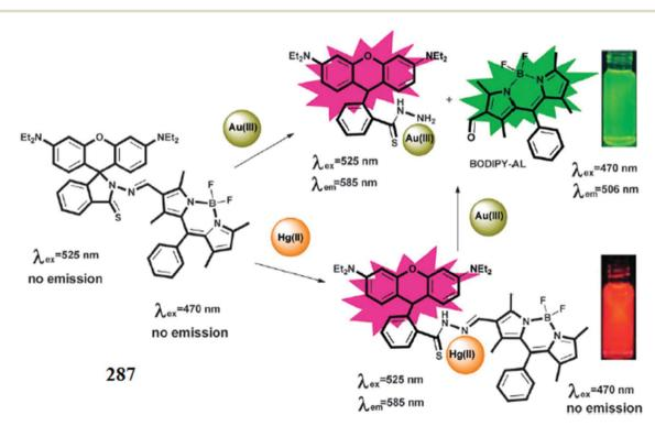
Fig. 251 Probe 287 and its response toward the addition of Au<sup>3+</sup> and Hg<sup>2+</sup>.
