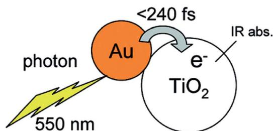
Fig. 3 Schematic representation of a gold nano dot attached on a  $\text{TiO}_2$  nanoparticle, also indicating hot electron transfer process upon the excitation of LSPR. Figure reprinted with permission from ref. 59.
