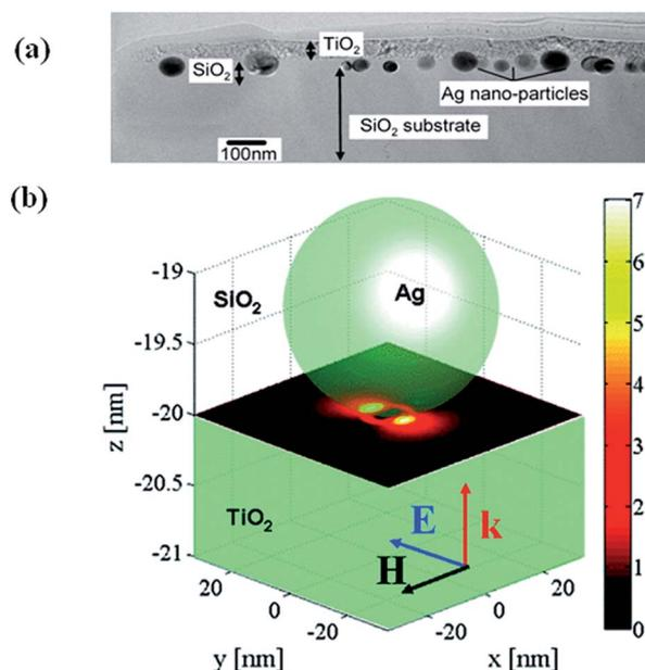
Fig. 4 (a) TEM cross sectional view showing  $\text{TiO}_2$  film on  $\text{Ag}/\text{SiO}_2$  core–shell on a  $\text{SiO}_2$  substrate. (b) Simulation showing the near-field amplitude enhancement inside a  $\text{TiO}_2$  substrate at the interface to a  $\text{SiO}_2$  substrate where a Ag NP is embedded. The  $y$ -polarized illuminating plane wave propagates in the  $z$ -direction. Reprinted with permission from ref. 56.
