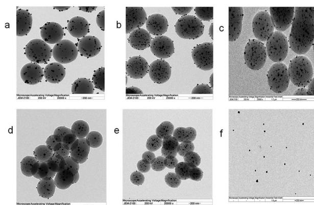
Fig. 9 TEM images, with 200 nm scale bar, of different sizes of poly-dopamine spheres loaded with silver nanoparticles (Ag@PDS) controlled by adjusting the amount of aqueous ammonia: (a) 1.0 ml, (b) 1.25 ml, (c) 1.5 ml, (d) 1.75 ml, (e) 2.0 ml and (f) pure Ag NPs. Ag@PDS of different sizes are applied in the antibacterial experiments.
