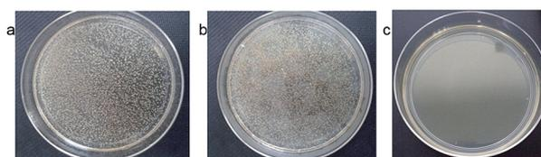
Fig. 10 Images of LB-agar plates used in the antibacterial experiments of samples against *E. coli*: (a) control, (b) poly-dopamine spheres (PDS), and (c) poly-dopamine spheres loaded with silver nanoparticles (Ag@PDS).
