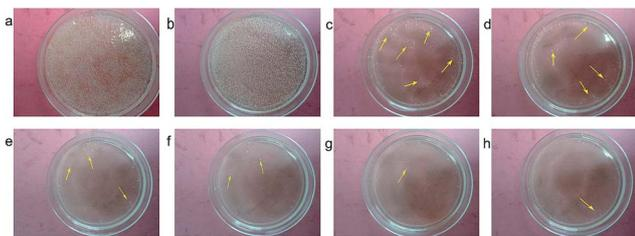
**Fig. 11** Antibacterial efficacy of samples against *S. aureus*. There is a robust growth of bacteria in images (a) and (b), while there are only a few surviving bacteria in (c)–(h). Samples: (a) control, (b) PDS, (h) pure Ag NPs, (c)–(g) Ag@PDSx with different amounts of aqueous ammonia: (c)  $x = 1.0$  ml; (d)  $x = 1.25$  ml; (e)  $x = 1.5$  ml; (f)  $x = 1.75$  ml; (g)  $x = 2.0$  ml.
