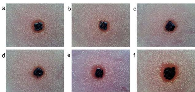
**Fig. 12** Disk diffusion tests for different samples against *S. aureus*. The zones of inhibition (ZOI) appear with an obvious circle, indicating a noticeable antibacterial effect. (a) Pure Ag NPs, (b)–(f) Ag@PDS with different amounts of aqueous ammonia: (b)  $x = 1.0$  ml; (c)  $x = 1.25$  ml; (d)  $x = 1.5$  ml; (e)  $x = 1.75$  ml; (f)  $x = 2.0$  ml.
