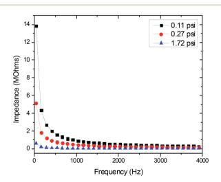
Fig. 2 Electrode-skin impedance with increasing application pressure.
