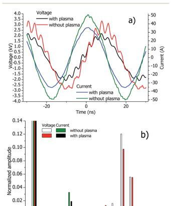
Fig. 3 Measured coil voltages and currents as functions of time (a) and their normalized Fourier spectra (b). The normalization makes the amplitudes of the fundamental wave of all the presented spectra equal to 1. A standard torch with optimal plasma conditions was used.
