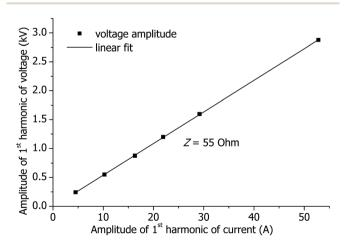
Fig. 2 Amplitudes of the  $1^{\rm st}$  harmonic of the measured voltage and current without plasma.
