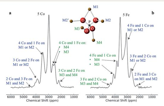
Fig. 6 Assignment of the peaks for (a)  $LiFe_{0.75}Co_{0.75}PO_4$  and (b)  $LiFe_{0.75}Co_{0.25}PO_4$ , using only the main contributions from the fittings. When Co is on M1 and/or M2, it results in lower shifts and placing a Co on M3 and/or M4 results in higher shifts. This is true for both materials.
