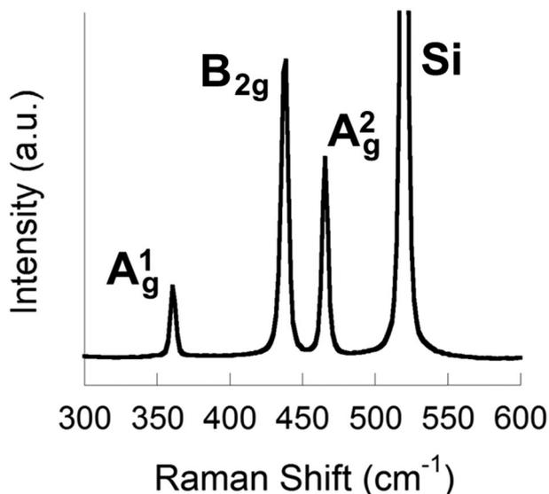
Fig. 2 Raman spectrum of few-layer phosphorene on a  $\text{SiO}_2/\text{Si}$  substrate from liquid exfoliation of black phosphorus in NMP showing the characteristic Raman bands at  $361 \text{ cm}^{-1}$ ,  $438 \text{ cm}^{-1}$  and  $465 \text{ cm}^{-1}$  assigned to the  $\text{A}_g^1$ ,  $\text{B}_{2g}$  and  $\text{A}_g^2$  modes.
