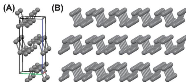
**Fig. 1** The chemical structures of the compounds in this study. (A) The orthorhombic unit cell of black phosphorus<sup>19</sup> ( $a = 3.31 \text{ \AA}$ ,  $b = 4.38 \text{ \AA}$ ,  $c = 10.50 \text{ \AA}$ ,  $\alpha = \beta = \gamma = 90^\circ$ ; space group *Bmab*; Crystallography Open Database ID: 1010325) which generates a layer structure comprising corrugated lamellae of phosphorus atoms held together by weak interlayer forces. (B) Three-layer phosphorene.
