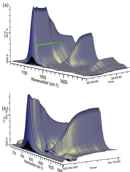
Fig. 2 *In situ* IR plots of the lithiation of **3a** with *n*-BuLi/(-)-sparteine at -78 °C in PhMe with time in h:min:s. (a)  $\nu_{\text{C=O}}$  **3a** (1691 cm<sup>-1</sup>), pre-mixed *n*-BuLi/(-)-sparteine added at time 16 min,  $\nu_{\text{C=O}}$  lithiated **3a** (1640 cm<sup>-1</sup>); (b)  $\nu_{\text{C=O}}$  **3a** (1691 cm<sup>-1</sup>) and (-)-sparteine then *n*-BuLi added at time 16 min,  $\nu_{\text{C=O}}$  lithiated **3a** (1640 cm<sup>-1</sup>).
