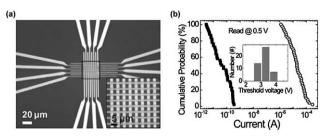
Fig. 19 (a) An optical image of a 2  $\mu$ m-scale memory device in an 8  $\times$  8 array structure. (b) A I-V curve of the 100 nm-scale device. Reproduced with permission.26 Copyright 2011, Wiley.
