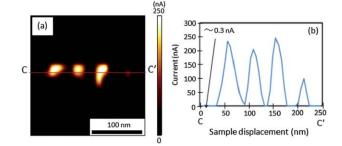
Fig. 20 (a) A conductive image of the PI film after dot pattern modification. (b) The current profile along C-C' in (a). Reproduced with permission.32 Copyright 2010, IOP Publishing Ltd.
