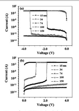
**Fig. 12** *I–V* curves of a Au/6F-2TPA PI/Al sandwich device using various thickness (15–150 nm) films; the voltage was swept to both (a) negative and (b) positive directions. Reproduced with permission. Copyright 2009, IOP Publishing Ltd.
