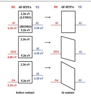
**Fig. 17** Energy level diagrams of 6F-HTPA PI and various electrodes. Reprinted with permission from ref. 15. Copyright 2009, American Chemical Society.
