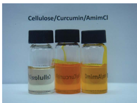
Fig. 2 The photographs of cellulose (left, 4%), curcumin (middle, 1%) and cellulose/curcumin solutions (right, 3% curcumin for cellulose) prepared with AmimCl solvent.
