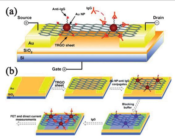
Fig. 14 (a) Schematic of the FET device. (b) Schematic illustration of the FET biosensor fabrication process. Reprinted with permission from ref. 509. Copyright 2010, John Wiley & Sons, Inc.
