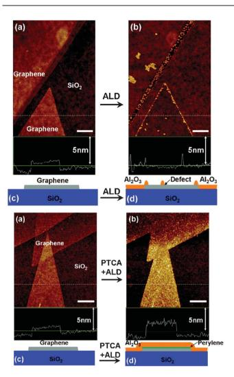
Fig. 7 ALD of Al<sub>2</sub>O<sub>3</sub> on (Top) pristine GN and (Bottom) PCTAcoated GN. (a) Atomic force microscopy (AFM) image of GN on SiO<sub>2</sub> before ALD. (b) AFM image of the same area as (a) after Al<sub>2</sub>O<sub>3</sub> ALD deposition. (c) and (d) Schematics of GN on SiO<sub>2</sub> before and after ALD. Reprinted with permission from ref. 330. Copyright 2008, American Chemical Society.
