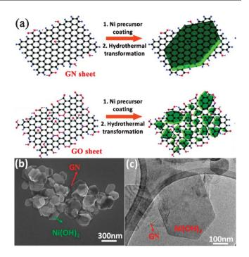
Fig. 5 (a) Schematic illustration of two-step Ni(OH)<sub>2</sub> nanocrystals hydrothermal growth on (top) GN and (bottom) GO sheets. (b) SEM and (c) TEM images of hexagonal Ni(OH)2 nanoplates formed on top of GN sheets. Reprinted with permission from ref. 306. Copyright 2010, American Chemical Society.
