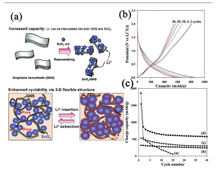
Fig. 13 (a) Schematic illustration for the synthesis and structure change of GN–SnO<sub>2</sub> nanocomposite during Li<sup>+</sup> insertion and extraction. (b) Charge–discharge profile for GN–SnO<sub>2</sub> nanocomposite. (c) Cyclic performances for (a) bare SnO<sub>2</sub> NPs, (b) graphite, (c) GN, and (d) GN–SnO<sub>2</sub> nanocomposite. Reprinted with permission from ref. 450. Copyright 2009, American Chemical Society.
