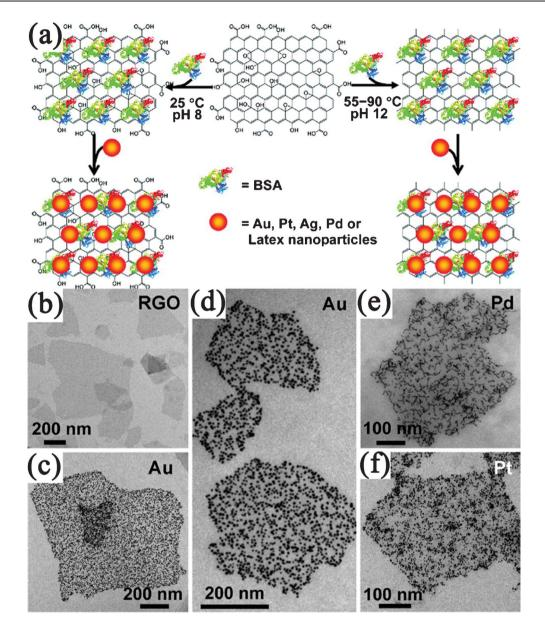
Fig. 9 (a) Illustration of assembly of noble metal NPs on GO/RGO nanosheets with the assistance of BSA. TEM images of (b) BSA–RGO nanosheets and BSA–RGO supported (c,d) Au, (e) Pd, and (f) Pt NPs. Reprinted with permission from ref. 345. Copyright 2010, American Chemical Society.
