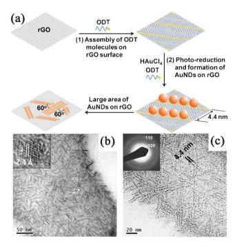
**Fig. 4** (a) Schematic illustration of the *in situ* synthesis and assembly of Au NDs on RGO. (b) TEM and (c) magnified TEM images of ODT-capped Au NDs synthesized *in situ* on RGO surface. Reprinted with permission from ref. 250. Copyright 2010, John Wiley & Sons, Inc.
