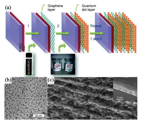
Fig. 3 (a) Fabrication of multilayered GN–CdS QDs nanocomposite. (b) TEM images of CdS QDs on GN nanosheets, (c) Cross-sectional scanning electron microscopy (SEM) image of a (GN–CdS QDs)<sub>10</sub> sample. The inset shows its thickness. Reprinted with permission from ref. 228. Copyright 2010, John Wiley & Sons, Inc.
