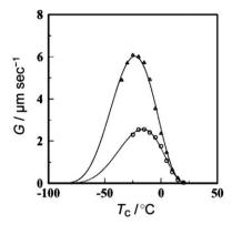
**Fig. 4** Crystallization temperature  $(T_c)$  dependence of spherulite growth rates (G) for linear  $(\triangle)$  and ring  $(\bigcirc)$  poly(THF)s.
