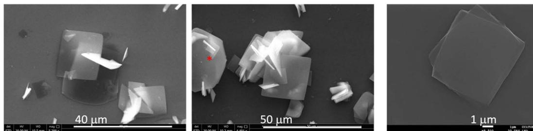
Fig. 2 SEM images for **1Si** (48 h deposition time) showing the growth of microcrystals from the functionalized Si. The EDS analysis corresponds to the flake with the red asterisk on the central image.
