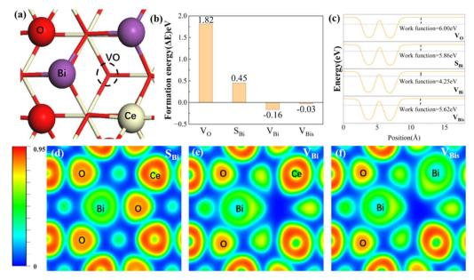
Fig. 1 (a) Configuration of four concept structures in CeO<sub>2</sub> (111). The formation energy (b), work function (c), and electron localization function (d-f) of the above four materials. White, red, and purple represent Ce, O, and Bi, respectively
