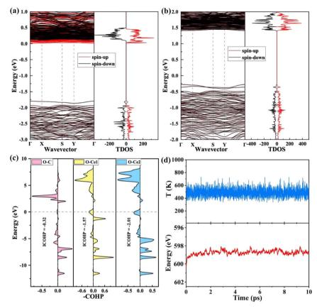
Fig. 3 Calculated electronic structures of  $V_{Bi}$  (a) and  $V_{Bis}$  (b). The Fermi energy is set as zero. (c) Projected crystal orbital Hamilton population (pCOHP) between O–C, O1–Ce1 and O2–Ce2. (d) Fluctuation of temperature and energy *versus* time (10 ps).
