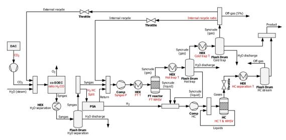
Fig. 2 Simplified process flow sheet of the PtL production evaluated in this study. Operation parameters which are varied during the process analysis described in this study are highlighted in red
