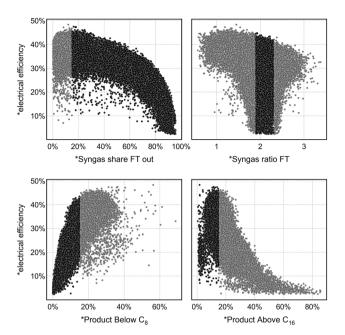
Fig. 6 Relationship between the four constrained process state parameters described in Section 2.2.6 and the achieved electrical efficiencies of all samples. Results that do not meet the constraints assumed in this study are displayed in grey. The resulting Pareto frontiers allow an assessment of the trade-offs in terms of electrical efficiency if the constraints are further narrowed.
