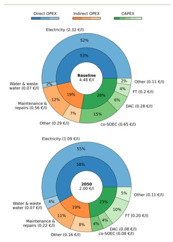
Fig. 7 Breakdown of the cost components of the NPC for the baseline scenario and the 2050 scenario (figures do not add up precisely due to roundina).
