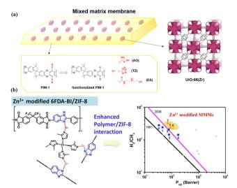
Fig. 14 (a) Combination of UiO-66(Zr) fillers and PIM-1 functionalized with AO, TZ and EA. Reproduced with authorisation from ref. 94 and copyright 2021 by American Chemical Society. (b) Metal-modified 6FDA-BI/ZIF-8 MMMs and separation performance comparison. Reproduced with authorisation from ref. 95 and copyright 2022 by
