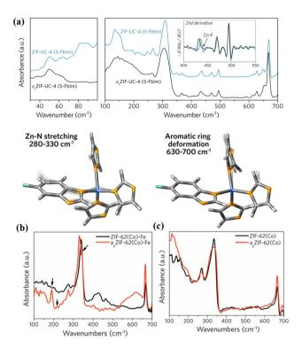
Fig. 7 (a) Structure comparison of MOF crystals and glass by THz/far-IR and the modes of ZnIm35-FbIm tetrahedra and aromatic rings utilized in DFT calculations. Reproduced with authorisation from ref. 65 and copyright 2020 by American Chemical Society. THz/Far-IR spectra of the vitrification for (b) ZIF-62(Co)-Fe and (c) ZIF-62(Co). Reproduced with authorisation from ref. 66 and copyright 2022 by Wiley-VCH GmbH.
