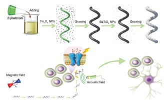
Fia. 3 The schematic diagram depicting the assembly S. platensis@Fe<sub>3</sub>O<sub>4</sub>@tBaTiO<sub>3</sub> micromotors, and the motors precisely stimulate the differentiation of neural stem cell-like cells under magnetic driving. This figure has been adapted from ref. 57 with permission from John Wiley and Sons, copyright 2020.
